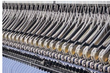
Weighting arms that require no compressed air
